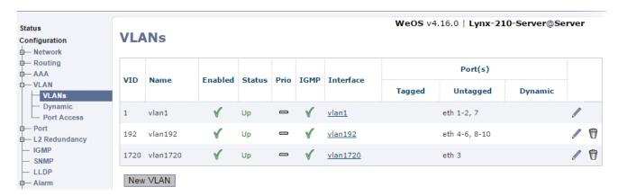
Client: VLAN 192 is the internal LAN and VLAN 1721 is the external WAN connection.
