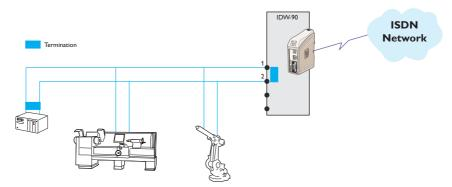
In this application the IDW-90 is set to communicate with a number of units with RS-485 interface. The communication is 2 wire half duplex at  $38\,400\,$  bit/s,  $8\,$  data, parity even and  $1\,$  stop bit.
